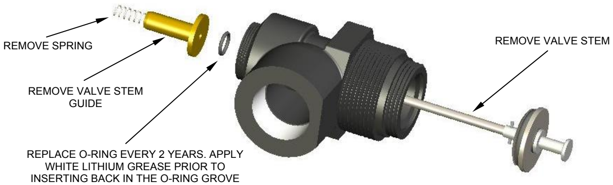
Figure 12H – STEP 7 – Replace valve seat and valve stem base o-rings.
