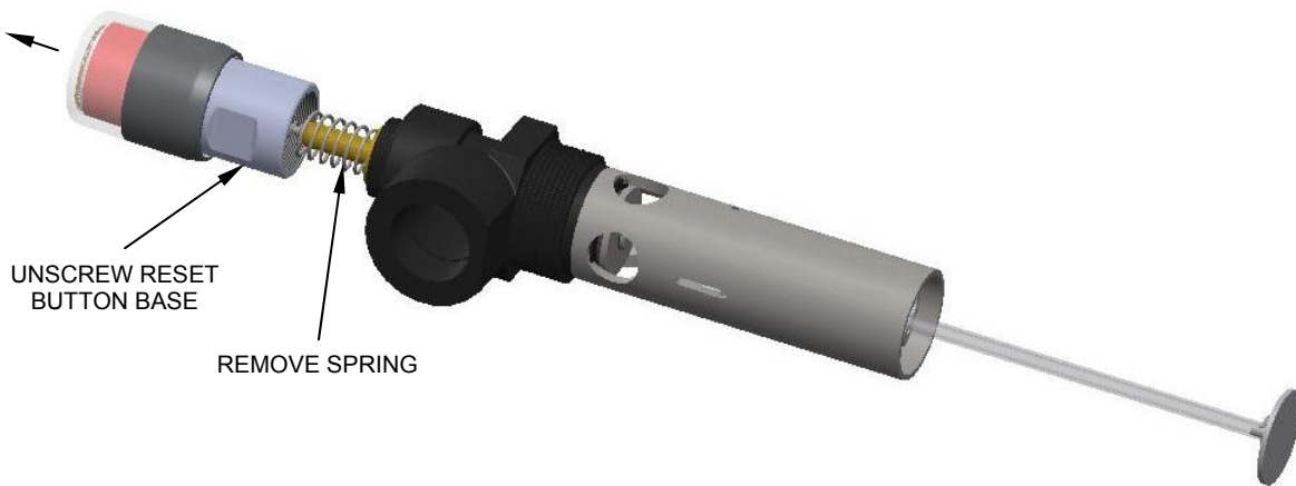
Figure 12B – STEP 2 – Unscrew reset button base and remove the spring
